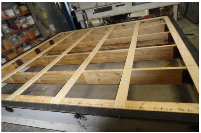
TEST ASSEMBLY F 1x4 WOOD PURLINS BEFORE TESTING
